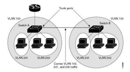
VLAN 100 = Primary VLAN VLAN 201 = Secondary isolated VLAN VLAN 202 = Secondary community VLAN
