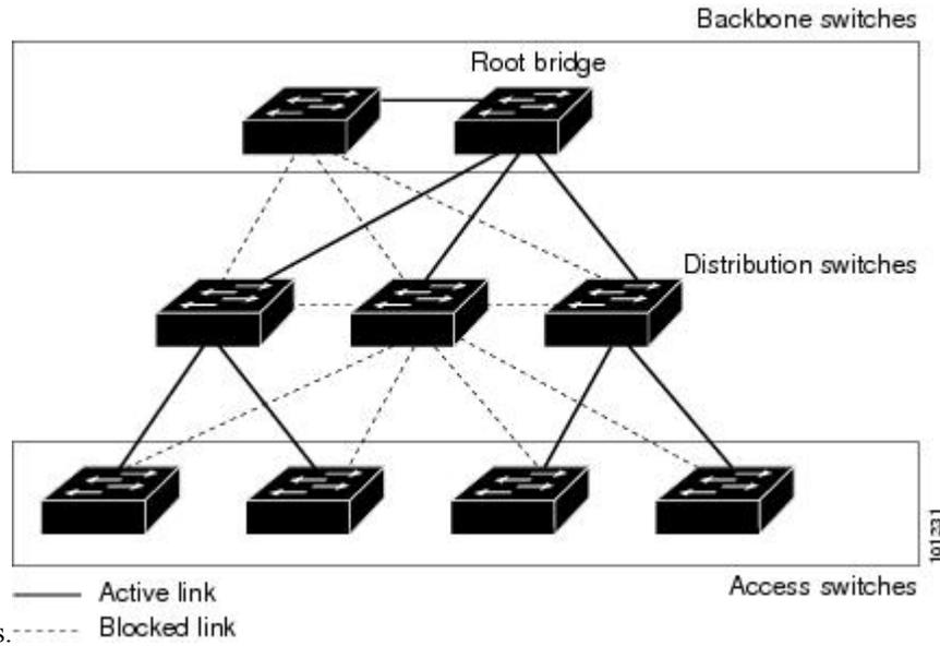
If a switch loses connectivity, it begins using the alternate paths as soon as the spanning tree selects a new root port. You can accelerate the choice of a new root port when a link or switch fails or when the spanning tree reconfigures itself by enabling UplinkFast. The root port transitions to the forwarding state immediately without going through the listening and learning states, as it would with the normal spanning-tree procedures.
