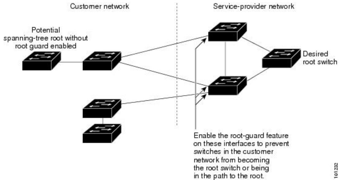
If a switch outside the SP network becomes the root switch, the interface is blocked (root-inconsistent state), and spanning tree selects a new root switch. The customer's switch does not become the root switch and is not in the path to the root.
