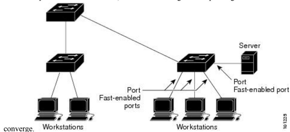
Interfaces connected to a single workstation or server should not receive bridge protocol data units (BPDUs). An interface with PortFast enabled goes through the normal cycle of spanning-tree status changes when the switch is restarted.
