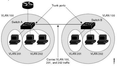
VLAN 100 = Primary VLAN VLAN 201 = Secondary isolated VLAN VLAN 202 = Secondary community VLAN
