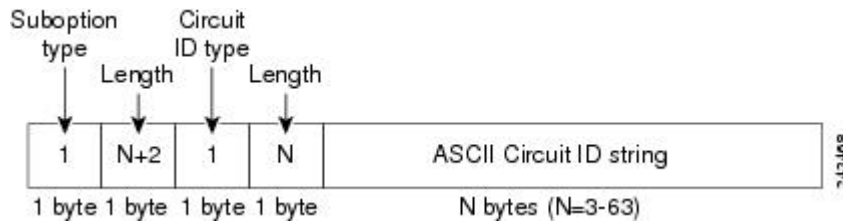
Figure 1: Suboption Packet Formats, Circuit ID Specified
