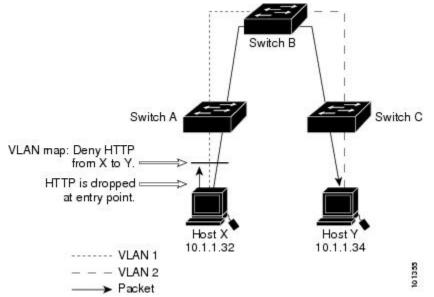
If you do not want HTTP traffic switched from Host X to Host Y, you can configure a VLAN map on Switch A to drop all HTTP traffic from Host X (IP address 10.1.1.32) to Host Y (IP address 10.1.1.34) at Switch A and not bridge it to Switch B.
