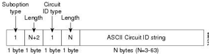
Figure 6: Suboption Packet Formats, Circuit ID Specified
