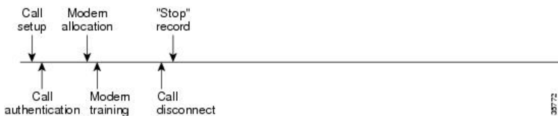
Figure 6: Modem Dial-In Call Setup Sequence With Call Disconnect Occurring Before User Authentication and With Resource Failure Stop Accounting Enabled
