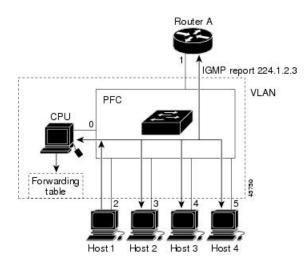
Router A sends a general query to the device, which forwards the query to ports 2 through 5, all of which are members of the same VLAN. Host 1 wants to join multicast group 224.1.2.3 and multicasts an IGMP membership report (IGMP join message) to the group. The device CPU uses the information in the IGMP report to set up a forwarding-table entry that includes the port numbers connected to Host 1 and to the router.
