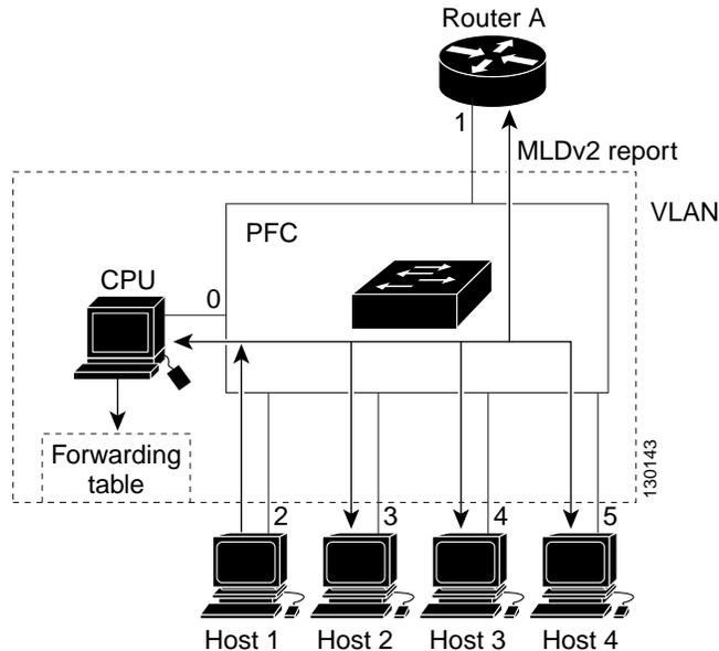
Multicast router A sends an MLD general query to the switch, which forwards the query to ports 2 through 5 (all members of the same VLAN). Host 1 wants to join an IPv6 multicast group and multicasts an MLD report to the group with the equivalent MAC destination address of 0x0100.5E01.0203. When the switch snoops the MLD report multicast by Host 1, the switch uses the information in the MLD report to create a forwarding-table entry.
