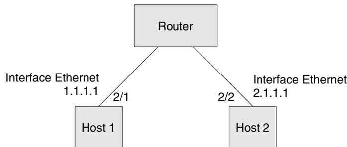
Physical Inter-VLAN Routing on a Catalyst 4500 series switch 94168
