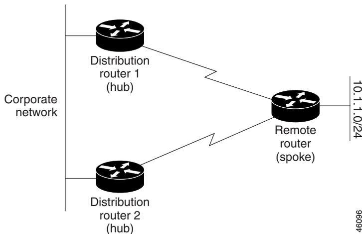
Figure 35-5 shows a simple dual-homed remote with one remote router and two distribution routers. Both distribution routers maintain routes to the corporate network and stub network 10.1.1.0/24.
