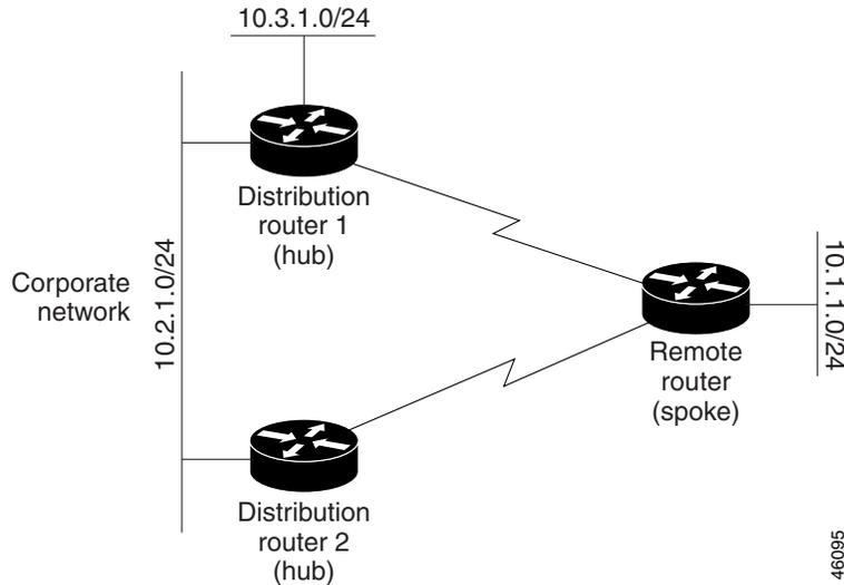
Figure 35-6 shows a simple dual-homed remote router where distribution router 1 is connected to both network 10.3.1.0/24 and network 10.2.1.0/24.
