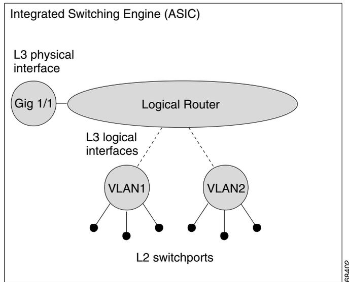
The Integrated Switching Engine performs inter-VLAN routing on logical Layer 3 interfaces with the ASIC hardware. The ASIC hardware also supports a physical Layer 3 interface that can be configured to connect with a host, a switch, or a router.
