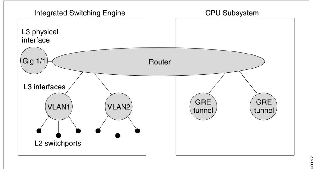
The Integrated Switching Engine performs inter-VLAN routing in hardware. The CPU subsystem software supports Layer 3 interfaces to VLANs that use Subnetwork Access Protocol (SNAP) encapsulation. The CPU subsystem software also supports generic routing encapsulation (GRE) tunnels.
