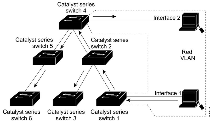
Figure 27-2 shows the same switched network with VTP pruning enabled. The broadcast traffic from Switch 1 is not forwarded to Switches 3, 5, and 6 because traffic for the Red VLAN has been pruned on the links indicated (Interface 5 on Switch 2 and Interface 4 on Switch 4).
