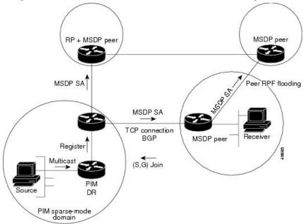
By default, the switch does not cache source or group pairs from received SA messages. When the switch forwards the MSDP SA information, it does not store it in memory. Therefore, if a member joins a group soon after an SA message is received by the local RP, that member needs to wait until the next SA message to hear about the source. This delay is known as join latency.
