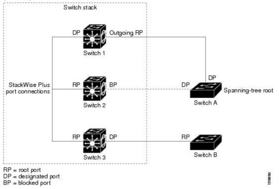
All paths that are not needed to reach the root device from anywhere in the switched network are placed in the spanning-tree blocking mode.
