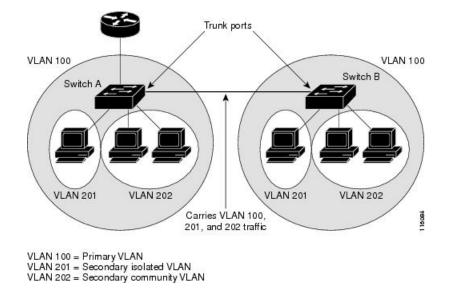
Private VLANs are supported in transparent mode for VTP 1, 2 and 3. Private vlan is also supported on server mode for VTP 3. If we have a server client setup using VTP 3, private vlans configured on the server should be reflected on the client.
