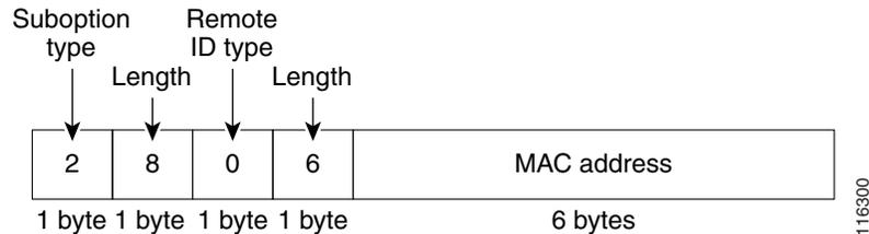
Figure 1-3 shows the packet formats for user-configured remote-ID and circuit-ID suboptions. The switch uses these packet formats when DHCP snooping is globally enabled and when the **ip dhcp snooping information option format remote-id** global configuration command and the **ip dhcp snooping vlan information option format-type circuit-id string** interface configuration command are entered.
