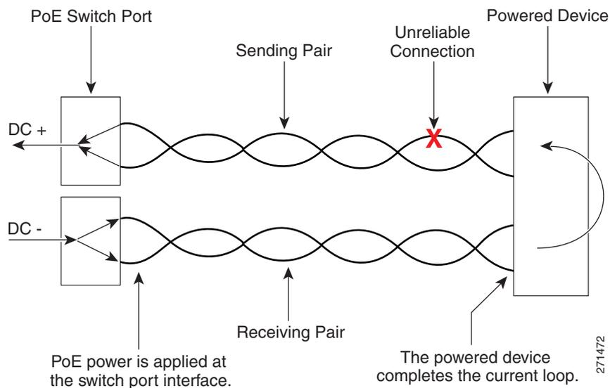
PoE requires both conductors of the send and receive pairs in order to deliver PoE power at 100 meters cable length, as shown in [Figure 5 on page 19](#). On shorter cables with one wire of the send or receive pair open, it might be possible to have powered device detection and classification, but no Ethernet link. On longer cables with an open wire in one of the pairs, it might not be possible to detect or power-up a powered device.
