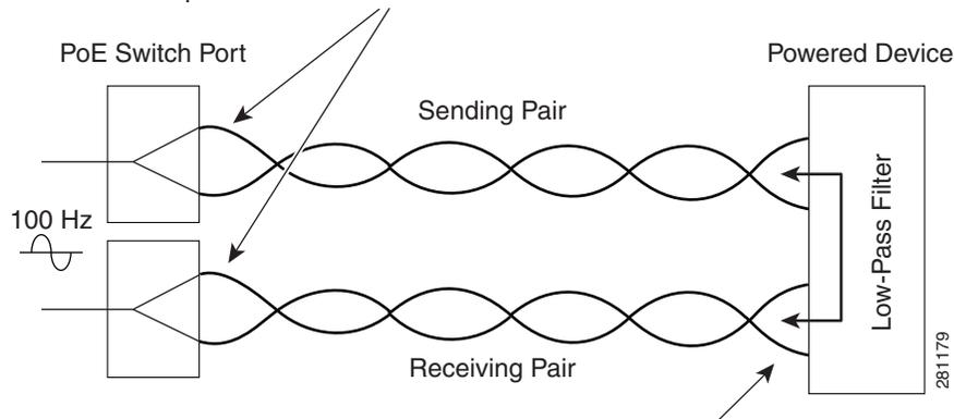
The low-pass filter provides a line termination at the signal frequency of 100 Hz.
