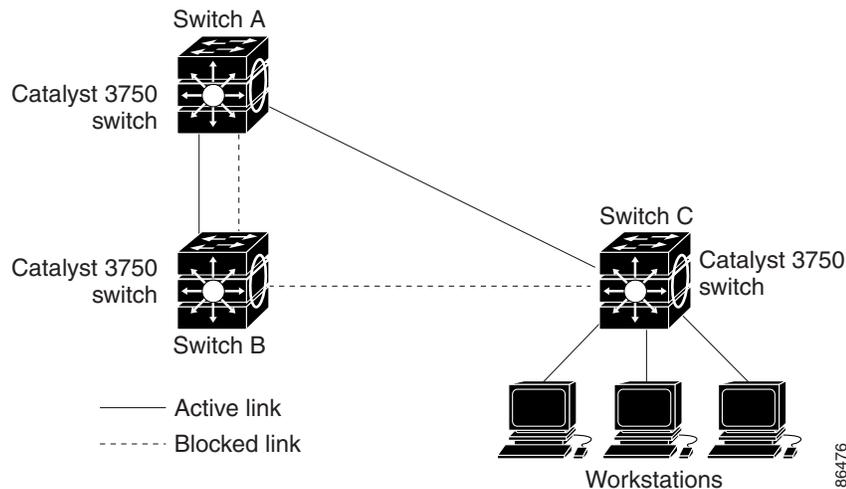
You can also create redundant links between switches by using EtherChannel groups. For more information, see the [Chapter 25, “Configuring EtherChannels.”](#)
