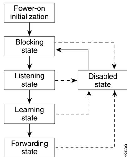
When you power up the switch, STP is enabled by default, and every interface in the switch, VLAN, or network goes through the blocking state and the transitory states of listening and learning. Spanning tree stabilizes each interface at the forwarding or blocking state.
