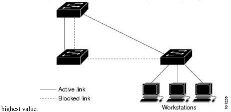
are the same, the port priority and port ID are added together, and spanning tree disables the link with the
