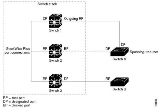
All paths that are not needed to reach the root device from anywhere in the switched network are placed in the spanning-tree blocking mode.
