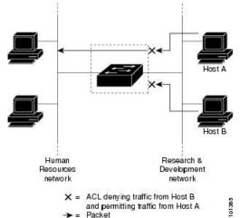
prevent Host B from accessing the same network. Port ACLs can only be applied to Layer 2 interfaces in the
