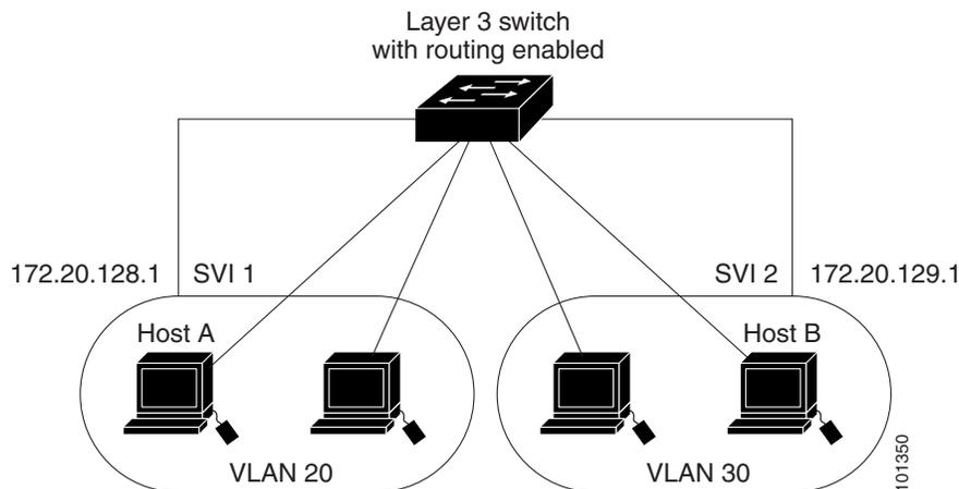
With the IP services image, the switch supports two methods of forwarding traffic between interfaces: routing and fallback bridging. With the IP base image, only basic routing (static routing and RIP) is supported. Whenever possible, to maintain high performance, forwarding is done by the switch hardware. However, only IP Version 4 packets with Ethernet II encapsulation can be routed in hardware. Non-IP traffic and traffic with other encapsulation methods can be fallback-bridged by hardware.
