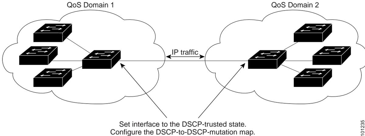
Beginning in privileged EXEC mode, follow these steps to configure the DSCP-trusted state on a port and modify the DSCP-to-DSCP-mutation map. To ensure a consistent mapping strategy across both QoS domains, you must perform this procedure on the ports in both domains:
