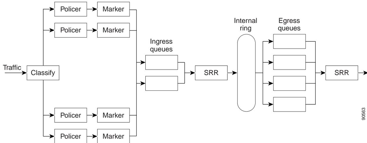
Because the total inbound bandwidth of all ports can exceed the bandwidth of the internal ring, ingress queues are located after the packet is classified, policed, and marked and before packets are forwarded into the switch fabric. Because multiple ingress ports can simultaneously send packets to an egress port and cause congestion, outbound queues are located after the internal ring.
