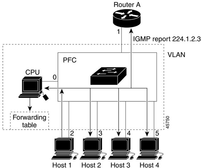
Router A sends a general query to the switch, which forwards the query to ports 2 through 5, which are all members of the same VLAN. Host 1 wants to join multicast group 224.1.2.3 and multicasts an IGMP membership report (IGMP join message) to the group. The switch CPU uses the information in the IGMP report to set up a forwarding-table entry, as shown in [Table 23-1](#), that includes the port numbers connected to Host 1 and the router.
