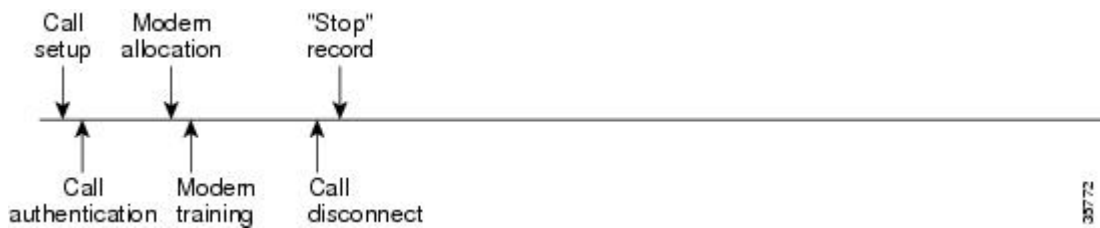
Figure 3: Modem Dial-In Call Setup Sequence With Call Disconnect Occurring Before User Authentication and With Resource Failure Stop Accounting Enabled
