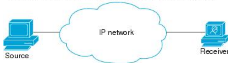
Unicast transmission—One host sends and the other receives.
