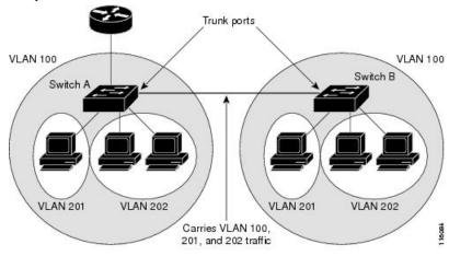
VLAN 100 = Primary VLAN VLAN 201 = Secondary isolated VLAN
