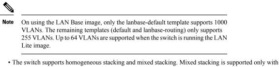
• The switch supports homogeneous stacking and mixed stacking. Mixed stacking is supported only with the Catalyst 2960-S switches. A homogenous stack can have up to eight stack members, while a mixed stack can have up to four stack members. All switches in a switch stack must be running the LAN Base image.
