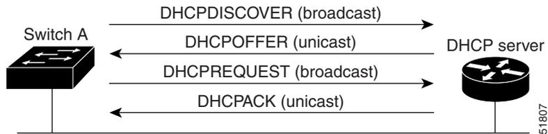
The client, Switch A, broadcasts a DHCPDISCOVER message to locate a DHCP server. The DHCP server offers configuration parameters (such as an IP address, subnet mask, gateway IP address, DNS IP address, a lease for the IP address, and so forth) to the client in a DHCPOFFER unicast message.
