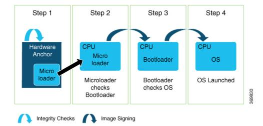
The public key, embedded directly into the hardware, is accessible via TAm libraries. Cisco IOS XE images are signed using private keys that are never removed from the build DevOps release environment. During the boot process, these keys are compared, confirming that both the hardware and software have been signed by Cisco.
