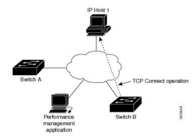
The connection response time is computed by measuring the time taken between sending a TCP request message from Switch B to IP Host 1 and receiving a reply from IP Host 1.
