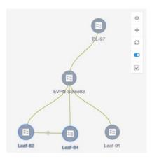
When you select multiple switches (Leaf-82 and Leaf-84 icons are highlighted in the example), the **Switches Deploy** screen for VRFs appears.
