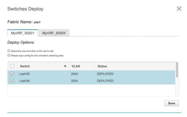
Each tab represents a VRF that you have chosen to undeploy (from the VRFs page). The tab contains a table. Each row in the table represents a switch on which the VRF has presence.
