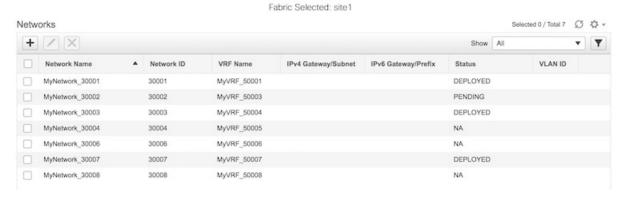
**Step 4** The delete button (**X**) is disabled by default. Select one or more networks you want to delete (by selecting appropriate check boxes). The delete button will be enabled. Click the delete button, and then click the Yes button that comes up to confirm network deletion.
