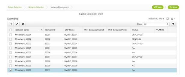
Step 2 Click Continue (on the top right part of the screen) to start deploying the network. If you also want to deploy other undeployed networks, select the appropriate check boxes and then click Continue.
