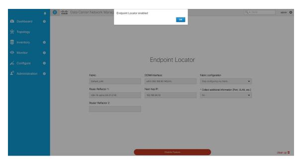
**Step 9** In case in Step 4, the "Configure my fabric" option is selected/checked, then the user has opted for the fully-automated mode for enabling EPL. Recall that in this case the DCNM server must be directly attached to a ToR/leaf switch. The appropriate connected switch and port on the other side of the DCNM *ethx* interface must be selected. The specified IP address will be configured on the selected interface on the connected switch.
