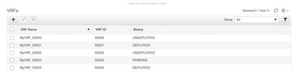
You can only undeploy VRF instances whose status is DEPLOYED. For example, you can undeploy MyVRF 50001 and MyVRF 50004.
