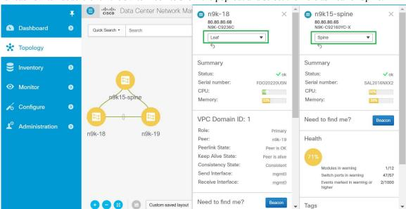
c) Set the role of the switches to Leaf or Spine as appropriate. To do so, access the Topology Display and for each switch double-click the switch-icon to show the pop-out and select the Role as Leaf or Spine.
