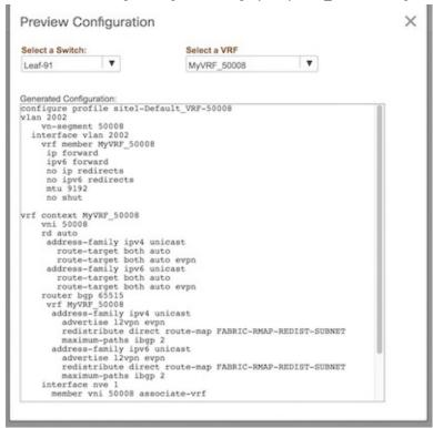
• Deployment - After you verify the configurations that are generated from the profiles are correct for the selected switches, click the **Deploy** button to deploy the configuration. DCNM will SSH to the switches and deploy the configuration. Then, DCNM shows the deployment status with the topology by highlighting the switches with different colors. You can also select the switch and view the deployment status details.
