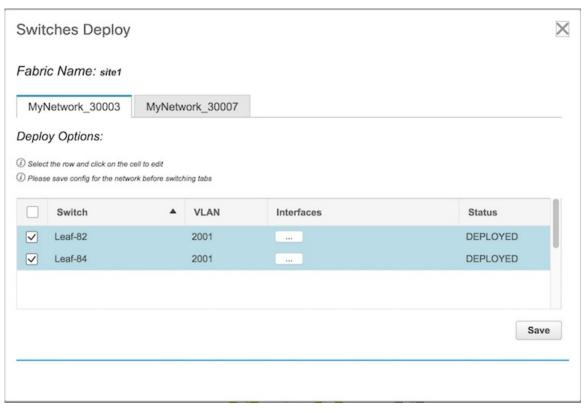
Each tab represents a network that you have chosen to undeploy (from the Networks page). The tab contains a table. Each row in the table represents a switch on which the network has presence.
