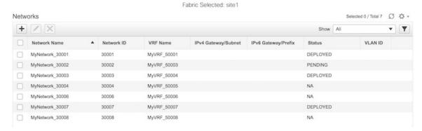
**Step 4** Select the networks you want to undeploy and click on the **Continue** button, at the top right part of the screen. The Topology screen comes up. This screen displays the fabric, the devices it is comprised of, and the connections between the devices.
