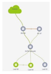
Different colors denote different statuses for the selected networks, as noted in the status panel at the bottom part of your screen. The deployed devices Leaf-82 and Leaf-84 are displayed in green color because the selected VRF instances are deployed on these devices.
