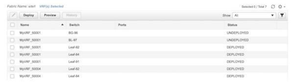
Select the appropriate network-switch combination and click the **Edit** button. The **Switches Deploy** screen comes up. Delete networks as per the process explained in the previous step.
