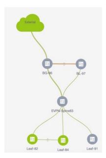
Different colors denote different statuses for the selected networks, as noted in the status panel. The deployed devices Leaf-82 and Leaf-84 are displayed in green color because MyNetwork\_30003 and MyNetwork\_30003 are deployed on these devices.
