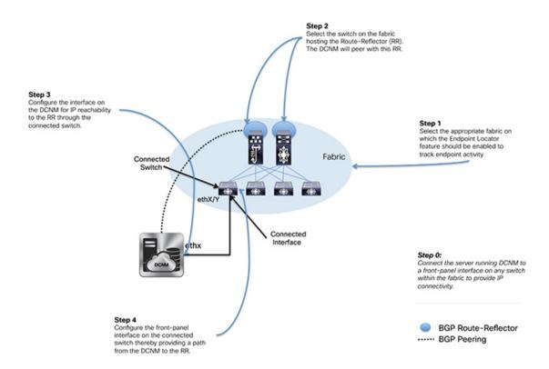
There are 2 sub-modes for configuring EPL which differ in how the network fabric will be configured to do BGP peering from the RR to the DCNM. These specifically differ in the options selected and entered in step 4. These sub-modes are:
