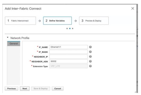
Here, the IP address details of the source and destination port are pre populated from the previous step. The template variables are parsed from the templates selected in the previous step and displayed for user input. All mandatory parameters must be entered.
