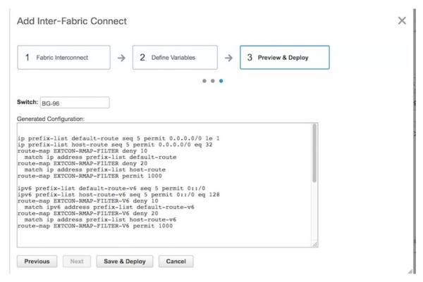
Here, you can preview the configuration that will be deployed to the selected border device. Note that no configuration will be pushed to the external device itself.
