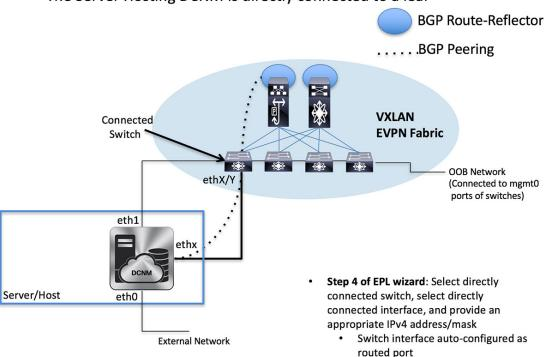
• **Semi-automated**—In this option, only the DCNM is configured appropriately for EPL. The assumption is that there is IP reachability already pre-established from the DCNM to the RR, hence an appropriate next-hop IP address should be provided in step 4 for this purpose. In addition, appropriate BGP neighborship configuration must be added to the RRs to accept DCNM as a peer. Note that, DCNM queries the BGP RR to glean information for establishment of the peering (e.g. ASN, RR IP etc.).
