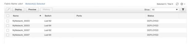
Select the appropriate network-switch combination and click the **Edit** button. The **Switches Deploy** screen will come up. Undeploy networks as per the process explained in the previous step.
