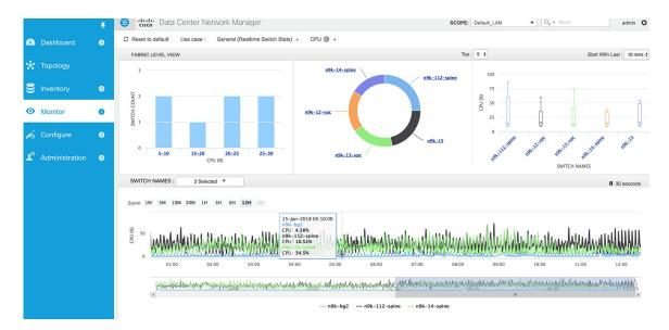
**Step 3** Every graph has a drill-down capability which enables the user to see the live CPU usage on a per switch per process basis. The per-process view can be triggered by simply clicking on the switch of interest in any of the graphs. Below is the drill-down view for the CPU metric with a sample selected switch (n9k-112-spine).
