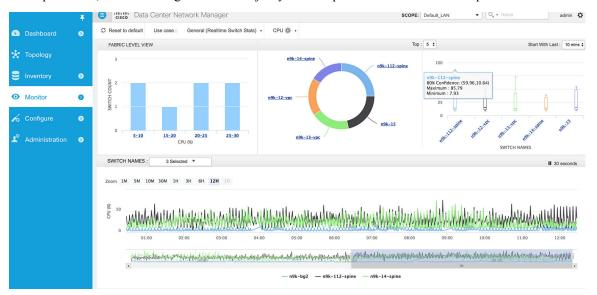
The representation at the bottom shows the real time CPU data feed for every switch. The graph refreshes automatically every 30 seconds. By default, 3 switches are selected to be displayed. The user can select up to a maximum of 5 switches by selecting them in the drop-down menu next to "SWITCH NAMES".
