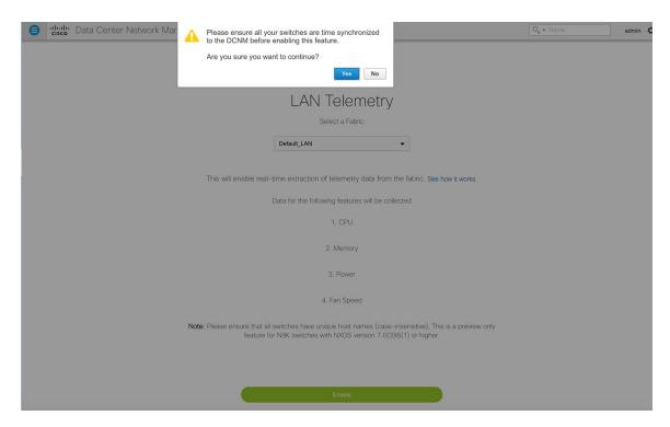
**Step 2** Once the feature is enabled, a message will appear indicating the initialization process has begun, which will take a couple of minutes. This time is needed for the streaming configuration to be pushed to the switches, the initial data to be streamed out from the switches, consumed by DCNM and depicted on the LAN telemetry dashboard.
