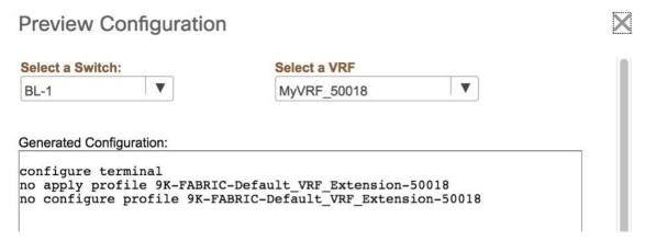
After you verify that the configuration profiles that will be removed are correct for the selected switches, click the **Deploy** button (on the top right part of the screen) to undeploy the MyVRF\_50018 and MyVRF\_50019 configurations on BL-1 and BL-2.
