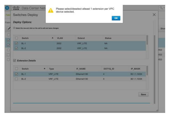
In the VRF extension on vPC switch pairs scenario, a tab is displayed for each VRF.
