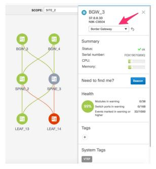
Likewise, update the role for BGW\_4 in site2 and then select site1 from the scope box and update roles for BGW 1 and BGW 2. This is required for configuring the EVPN Multi-Site feature through the DCNM GUI.
