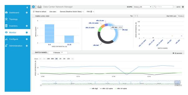
The drill down view provides the fan speed as a percentage metric of each individual fan within a selected device. A sample drill-down view for a selected device is shown below (n9k-bg1):
