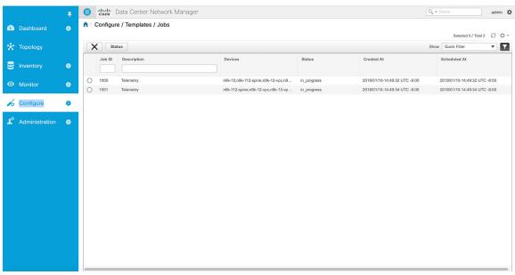
Once the jobs are successfully executed, the required telemetry configuration has been applied to the switches and the streaming data will appear once received and processed.
