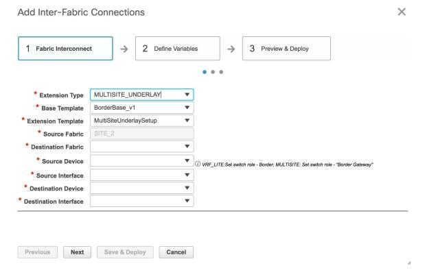
**Base Template**—By default, the BorderBase\_v1 base template is populated. This template is a one-time configuration pushed to the BGW.
