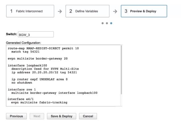
Here, you can preview the configuration that will be deployed to BGW\_3. Note that no configuration will be pushed to the external device itself.
