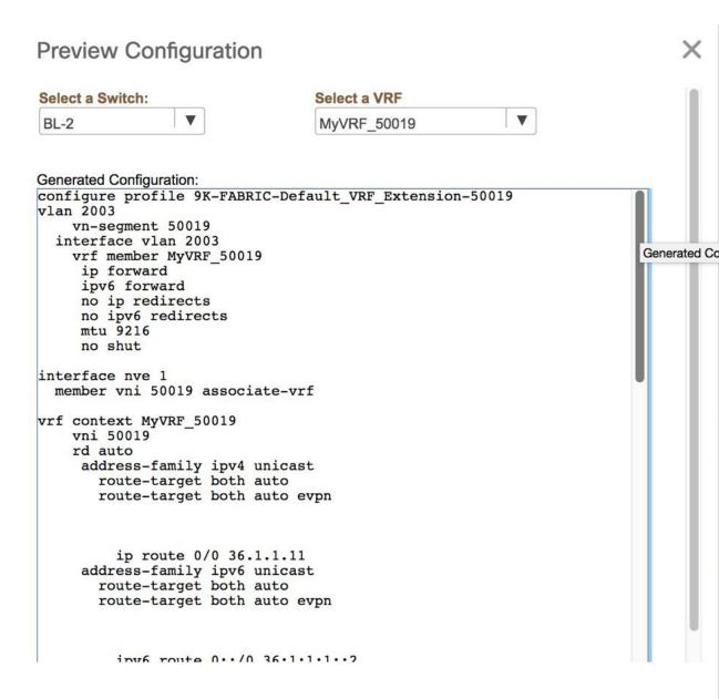
You can select a switch and a VRF to view corresponding configurations. Configuration details of MyVRF\_5016 that is pushed to BL-1 are included in the *Appendix* section.
