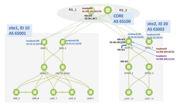
Network configurations for the two fabrics are provisioned through DCNM software, 10.4(2) release. VXLAN BGP EVPN configurations are configured on the switches in the two fabrics. However, server traffic between the sites is only possible through a Data Center Interconnect (DCI) function. If a server in site1 has to send
