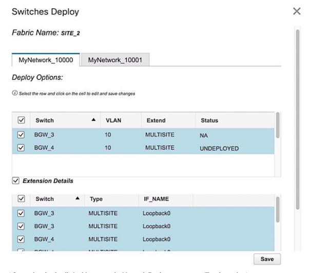
After saving the details in this screen, the Network Deployment screen (Topology view) appears.
