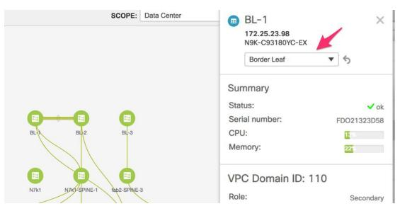
This is required for configuring the VRF Lite feature through the DCNM GUI. After completing the VRF Lite specific prerequisites, start DCNM VRF Lite configuration on BL-1 with extensions to the edge router ER-1.
