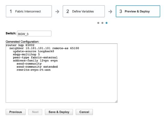
Here, you can preview the overlay configuration that will be deployed to BGW\_3. In this section, you can see that an overlay connection is being established from Loopback0 on BGW\_3 to the neighbor with AS Number 65100.
