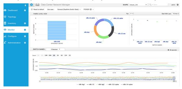
The drill down view indicates the input power in Watts, consumed by the individual power supply of the selected switch. A sample drill-down view for a selected device is shown below (n9k-112-spine):
