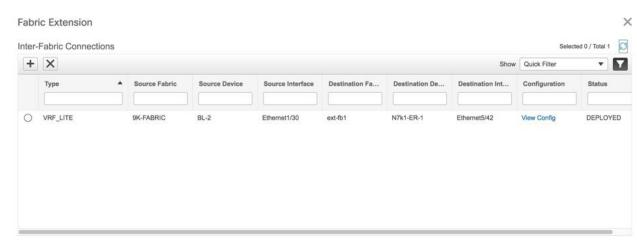
Similarly, select BL-2 and click **X** to remove the BL-2 inter-fabric connection. After both BL-1 and BL-2 VRF Lite inter-fabric connections are removed, the Fabric Extension screen will have no entries.
