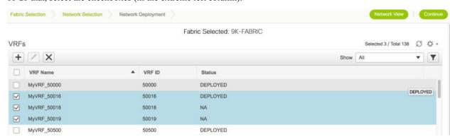
Click the **Continue** button at the top right part of the screen. The VRF Deployment page (Topology View) comes up. You can deploy VRFs on multiple switches simultaneously, but with the same role. So, deploy the selected VRFs on the border leafs.
