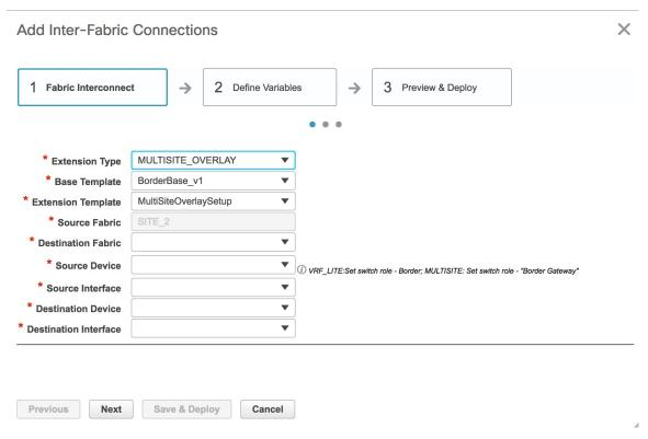
**Base Template**—*BorderBase\_v1* is auto-populated in this field. The *BorderBase\_v1* base template is a one-time configuration pushed to the BGW.
