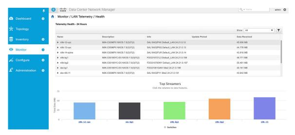
The bar graph depicts the top 5 streaming switches and a has drill-down capability for feature-wise break-down.
