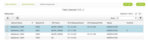
Click the **Continue** button at the top right part of the screen. The Network Deployment page (Topology View) comes up. You can deploy networks on multiple switches simultaneously, but with the same role. So, deploy the selected networks on the BGWs.
