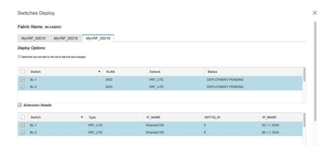
Click the **Save** button at the bottom right part of the Switches Deploy screen to save all VRFs' configurations on the selected switches. The VRF Deployment screen (Topology view) appears.
