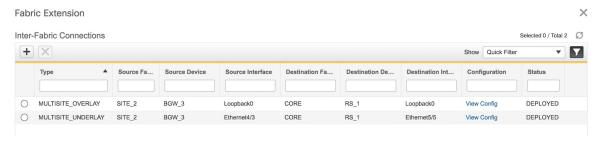
The view doesn't auto-refresh, hence the refresh button on the top right part of the screen needs to be clicked to trigger refresh. You can check the status of the deployment (Pending, Deployed, Failed) in the **Status** column. In case of FAILED or UNDEPLOYMENT FAILED status, use the hyperlink in the **Status** column to check the error messages for failure.
