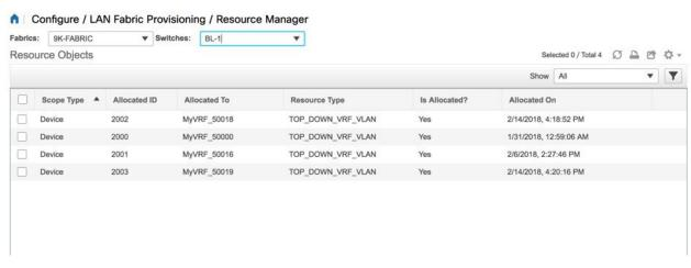
The VRF instances MyVRF\_50016, MyVRF\_50018, and MyVRF\_50019 are deployed on BL-1, with their corresponding VLANs 2001, 2002, and 2003.
