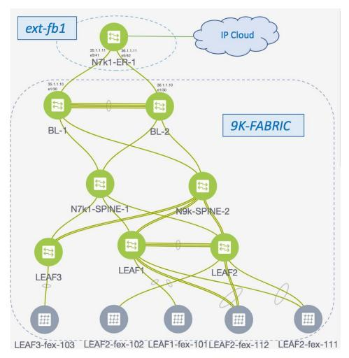
Network configurations for the fabric is provisioned through DCNM. For external Layer 3 reachability from hosts connected to leaf switches within the fabric, border devices need to be provisioned with the appropriate VRF configuration. Multiple border devices in the fabric ensure redundancy in the case of failures as well as effective load distribution.
