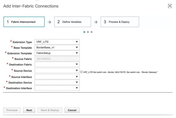
By default, VRF\_LITE is populated in the **Extension Type** field. Since the inter-fabric extension is through VRF Lite, retain this entry.
