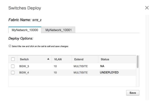
A tab is displayed for each network. Click the checkbox next to the **Switch** column. Both the BGW check boxes will be selected automatically and the **Extension Details** section will appear at the bottom part of the screen.
