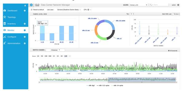
The middle tile depicts the Top 5 switches in the fabric with respect to average CPU usage. The user can select the Top 10 or Top 15 switches by choosing the drop-down menu above the middle tile.
