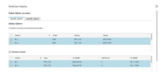
Double click the checkbox next to the Switch column or uncheck the check box next to BL-1 and BL-2. Both of the check boxes will be de-selected and the Extension Details section will disappear at the bottom part of the screen.
