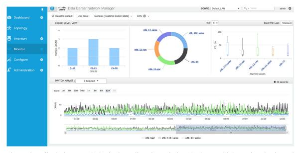
The top three tiles in the screen depict the data collected over the last 10 minutes. This interval can be changed by selecting a different time scale in the pull down. Next, we will describe the details depicted in the various tiles and graphs. The first tile on the left shows a fabric level view; it's a histogram showing the count of switches that fall within a certain CPU range.
