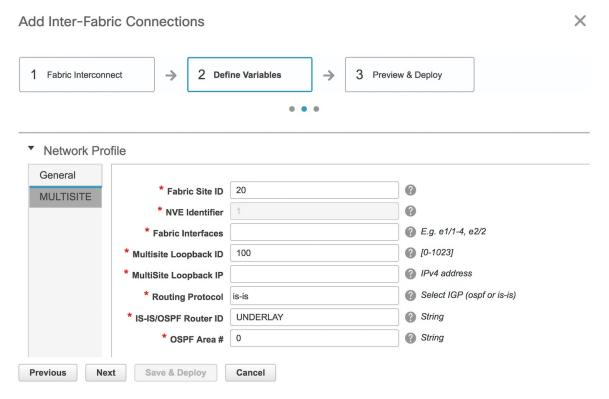
**Fabric Site ID**—This is the identification for the VXLAN BGP EVPN fabric site2 to which BGW\_3 belongs. When you configure the EVPN Multi-Site feature on BGW\_4 (or any other BGW on site2), the site ID will be 20. The site *site1* will be assigned with a unique ID.
