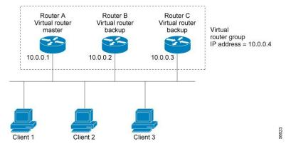
Because the virtual IP address uses the IP address of the physical Ethernet interface of Router A, Router A is the master (also known as the IP address owner). As the master, Router A owns the virtual IP address of the VRRP group and forwards packets sent to this IP address. Clients 1 through 3 are configured with the default gateway IP address of 10.0.0.1.
