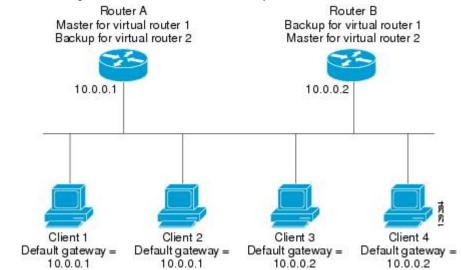
This topology contains two virtual IP addresses for two VRRP groups that overlap. For VRRP group 1, Router A is the owner of IP address 10.0.0.1 and is the master. Router B is the backup to Router A. Clients 1 and 2 are configured with the default gateway IP address of 10.0.0.1.
