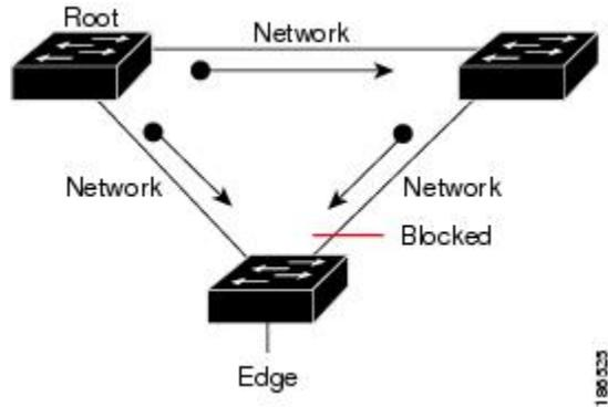
This figure demonstrates a potential network problem when the device fails and you are not running Bridge Assurance.
