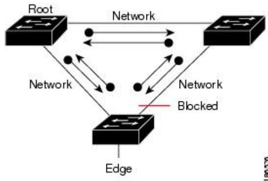
This figure shows how the potential network problem does not happen when you have Bridge Assurance enabled on your network.
