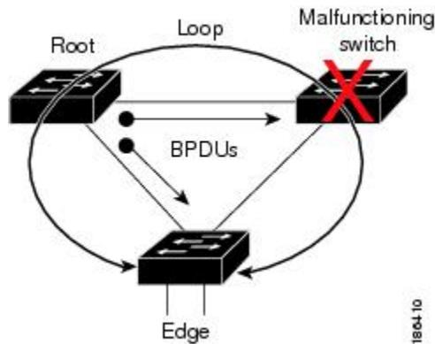
This figure shows the network with Bridge Assurance enabled, and the STP topology progressing normally with bidirectional BPDUs issuing from every STP network port.
