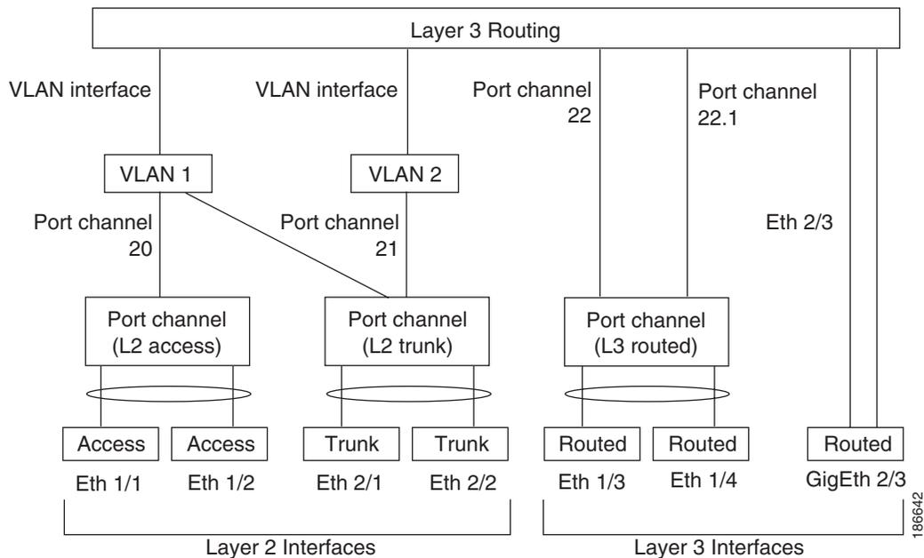
You can classify port-channel interfaces as Layer 2 or Layer 3 interfaces. In addition, you can configure Layer 2 port channels in either access or trunk mode. Layer 3 port-channel interfaces have routed ports as channel members and may have subinterfaces.
