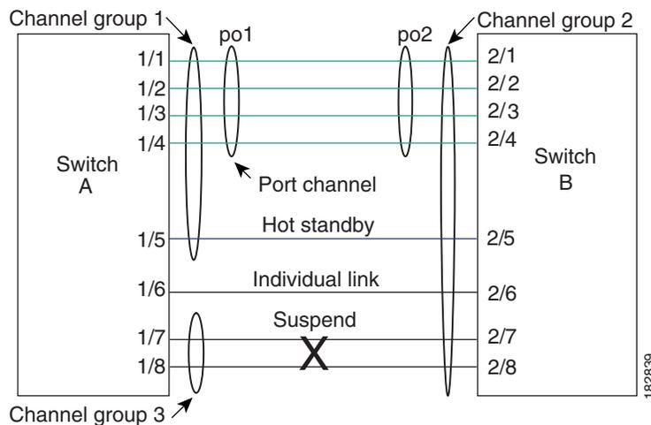
With LACP, you can bundle up to 16 interfaces in a channel group. If the channel group has more than eight interfaces, the remaining interfaces are in hot standby for the port channel associated with this channel group.
