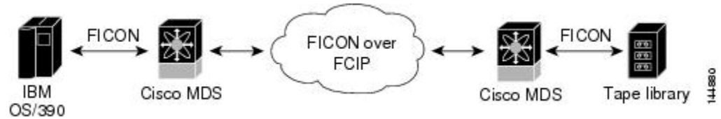
Figure 6: Host Accessing Standalone IBM-VTS (Virtual Tape Server)/STK-VSM (Virtual Shared Memory)
