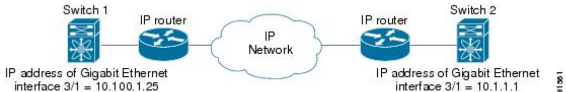
Figure 5: Assigning Profiles to Each Gigabit Ethernet Interface
