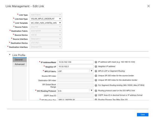
**IP** address/Mask: Specifies the IP address with mask for the source interface.
