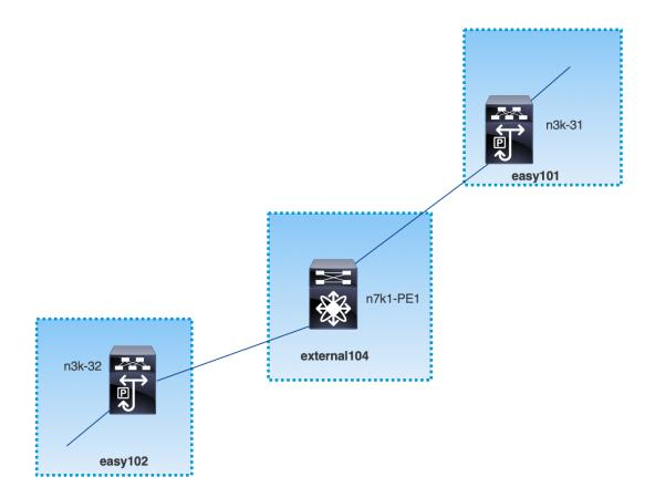
This topology shows only the border devices in the Easy Fabric and the core or edge router in the external fabric.
