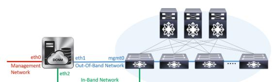
The following figure shows the network diagram for the Cisco DCNM Management interfaces.
