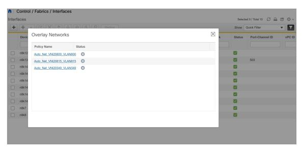
These are the networks that are attached to the **Ethernet 1/5** interface.
