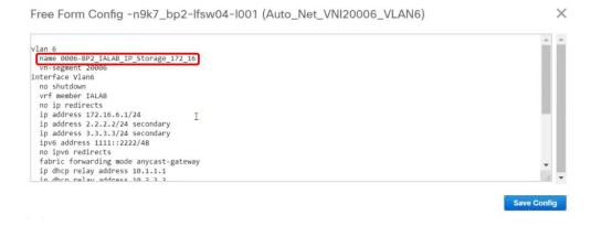
Step 8 Modify the VLAN name in the Free Form Config window and click Save Config.
