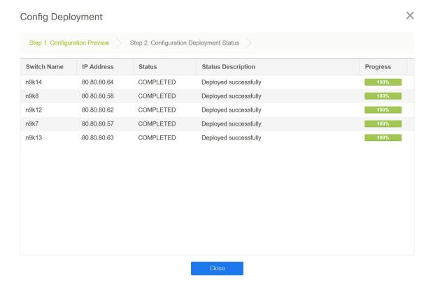
If the **Status** column displays **FAILED**, investigate the reason for failure to address the issue.
