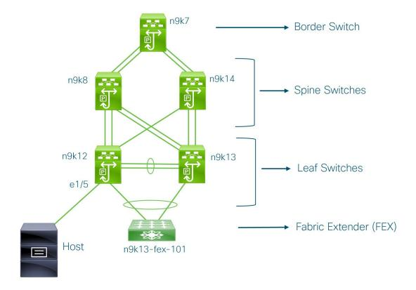
You can see that there is a border switch, two spine switches, two leaf switches, and a Fabric Extender or FEX.
