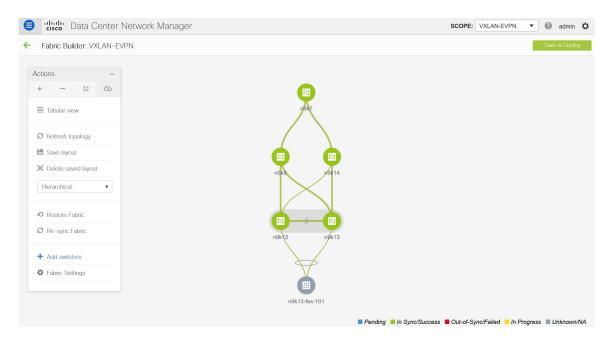
**Post-transitioning of VXLAN fabric management to DCNM** - This completes the transitioning process of VXLAN fabric management to DCNM. Now, you can add new switches and provision overlay networks for your fabric. For details, refer the respective section in the Fabrics topic in the configuration guide.
