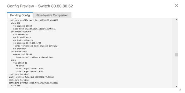
As part of the import process, after the configuration profiles are applied, the original CLI based configuration references will be removed from the switches. These are the 'no' CLIs that will be seen towards the end of the diffs. The VXLAN configurations on the switches will be persisted in the configuration profiles. In the following image, you can see that the configurations will be removed, specifically, **no vlan 160**.
