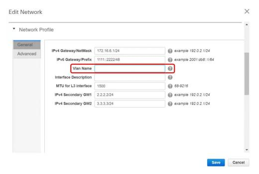
In the **Edit Network** window, the **Vlan Name** field is empty because DCNM has not captured this info in the overlay profile. Instead, the VLAN name is captured in the freeform config associated with the overlay network or VRF.
