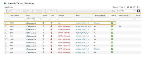
This interface is attached to the host through the n9k-12 switch.
