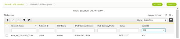
This network is associated with the VLAN ID 349 and is configured with the anycast IP 204.90.140.134.
