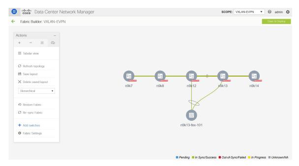
The switch discovery process might fail for a few switches, and the Discovery Error message is displayed. However, such switches are still displayed in the fabric topology. You should remove such switches from the fabric (Right-click the switch icon and click **Discovery** > **Remove** from fabric), and import them again.
