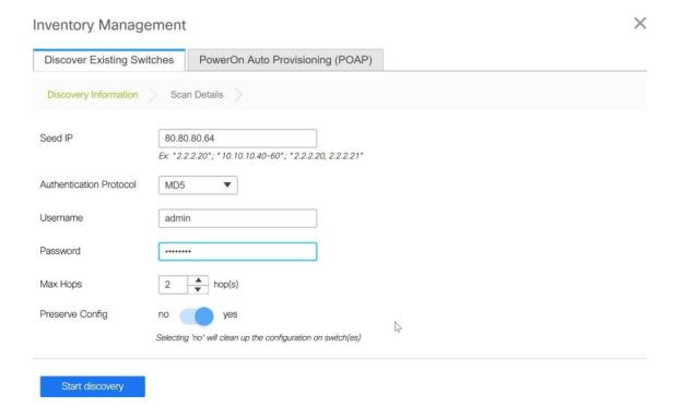
By default, the value in the **Max Hops** field is **2**. The switch with the specified IP address and the switches that are 2 hops from it will be populated after the discovery is complete.
