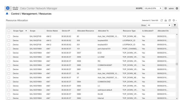
The resources that are being utilized by the VXLAN EVPN fabric such as VLAN IDs, port channel IDs, point to point IP addresses, and loopback IDs are displayed in this window.
