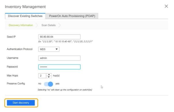
The switch with the specified IP address and switches up to two hops away (depending on the setting of Max Hops) from it are populated in the Scan Details section.
