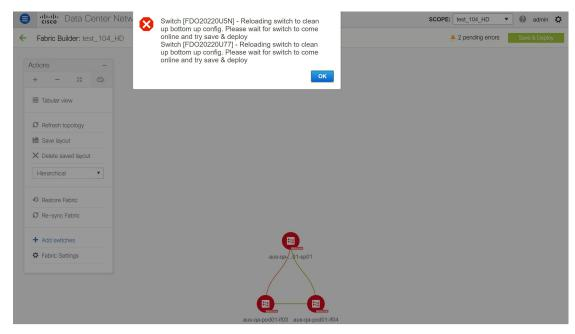
**4.** Wait for the switches to complete the reload operation. Click **Tabular view** under the **Actions** menu to view the status of the switches.
