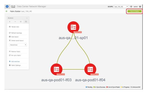
If the added switches contain bottom-up configurations, an error is displayed saying – Reloading switch to clean up bottom up config. Please wait for switch to come online and try **Save & Deploy**.
