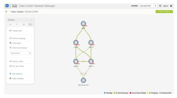
**vPC Pairing** - The vPC pairing must be done for switches where the Layer 3 vPC peer-keep alive is used. The vPC configuration is automatically picked up from the switches when the vPC peer keep alive is established through the management option. This pairing reflects in the GUI only after the migration is complete.
