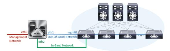
During Cisco DCNM installation for your deployment type, you can configure these interfaces. However, from Cisco DCNM Release 11.2(1), you can edit and modify the network settings post installation.
