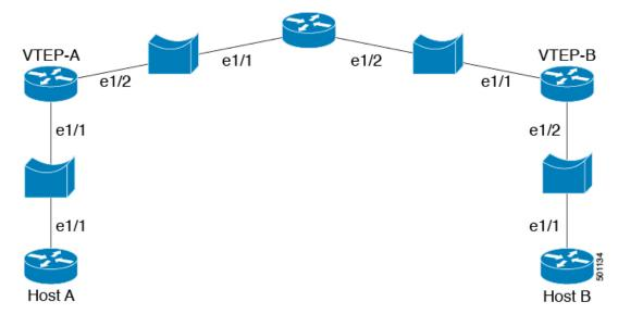
This topology can simulate basic vxlan functionality on Cisco Nexus 9000v platform. Similar bridge/vSwitch setup should be done as shown in other topology examples.
