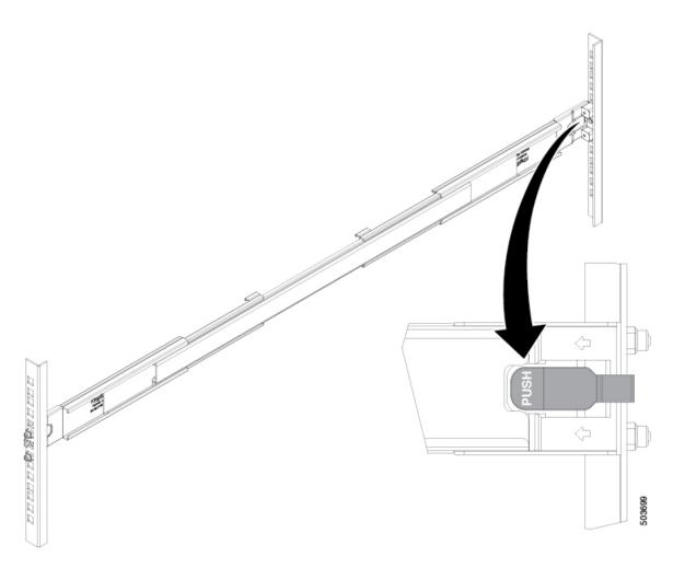
**Step 6** If installing from the front of the rack, slide the chassis into the rack by aligning the inner rails into the outer rails and sliding the chassis back until the front panel is flush with the front of the rack. Then secure the retainer screws on the inner rails into the rack, as shown.
