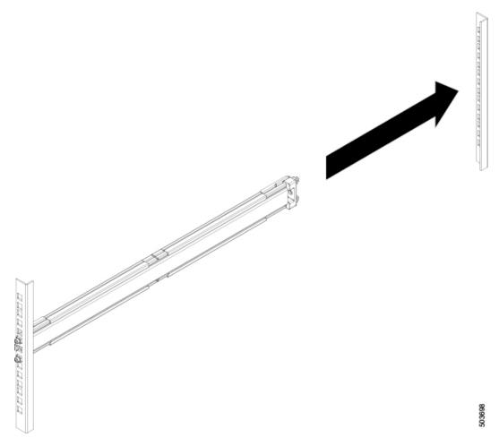
**Step 5** Fasten the two outer rails to the back posts of the rack by pushing the latch into place, as shown.
