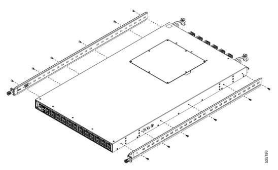
**Step 2** Install the two outer rails to the front posts of the rack by aligning the rails to the post holes, as shown.
