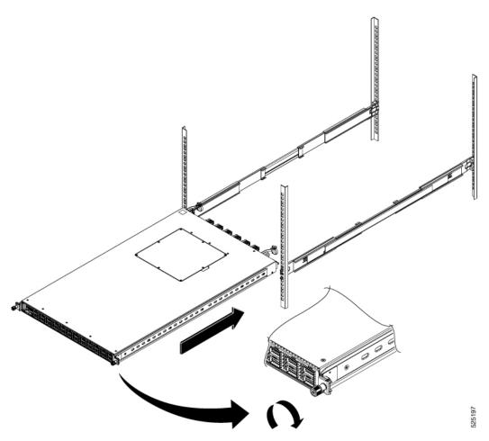
Step 7 If installing from the back of the rack, slide the chassis into the rack by aligning the inner rails into the outer rails, and sliding the chassis forward until the front panel is flush with the front of the rack. Then slide the retainer screws out to align with the rack and then secure the thumb-screws on the inner rails into the rack, as shown.
