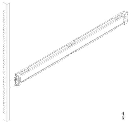
**Step 3** Fasten the two outer rails to the front posts of the rack by pushing the latch into place, as shown.
