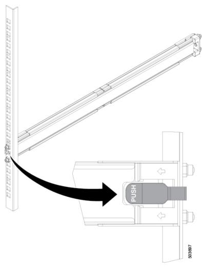
**Step 4** Install the two outer rails to the back posts of the rack by extending them into place, as shown.
