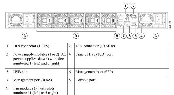
The following figure shows the switch features on the side of the chassis.
