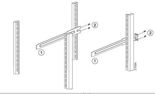
Slider rail with screw holes aligned to screw holes in rack
