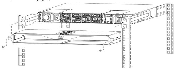
c) Tighten the 10-32 screws to 20 in-lb (2.26 N·m) or tighten the 12-24 screws to 30 in-lb (3.39 N·m).
