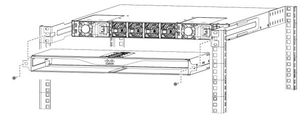
c) Tighten the 10-32 screws to 20 in-lb (2.26 N m) or tighten the 12-24 screws to 30 in-lb (3.39 N m).
