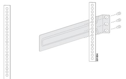
c) Repeat Step 3 to attach the other slider rail to the other side of the rack.
