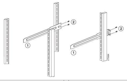
Slider rail with screw holes aligned to screw holes in 2 Two customer-supp to attach each slider
