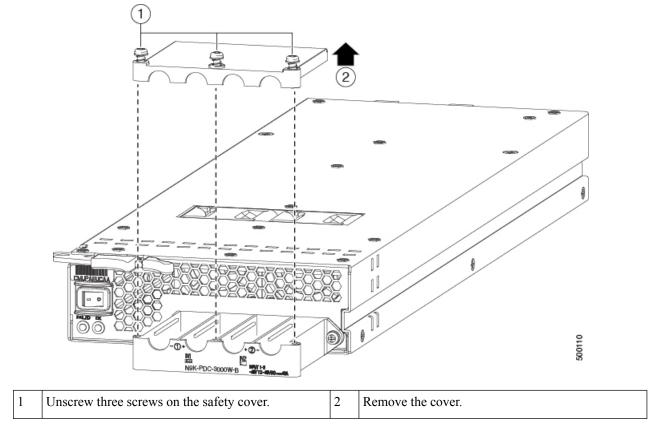
Note The terminal box has four slots for four power terminals (ordered as negative [-], positive [+], and negative [-]). Each terminal has two nuts that you use to fasten a power cable to the terminal.
