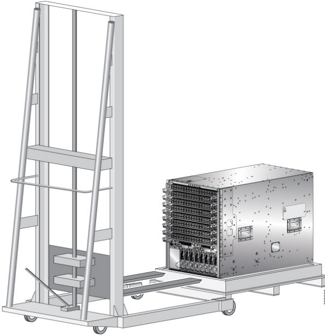
Figure 2: Align the Lifting Device in Front of the Chassis on the Pallet
